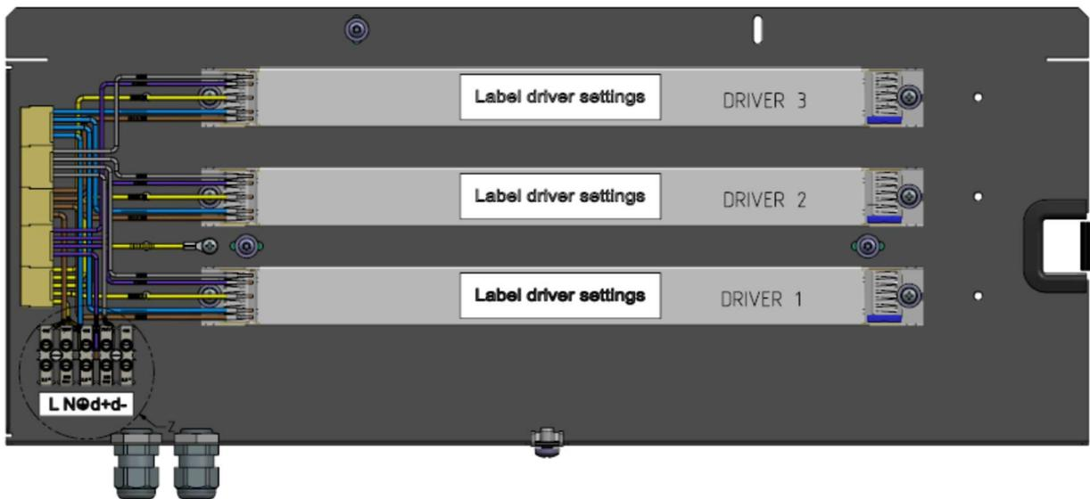
**Figure 4: Inside look of an E-box with the maximum quantity of drivers**
