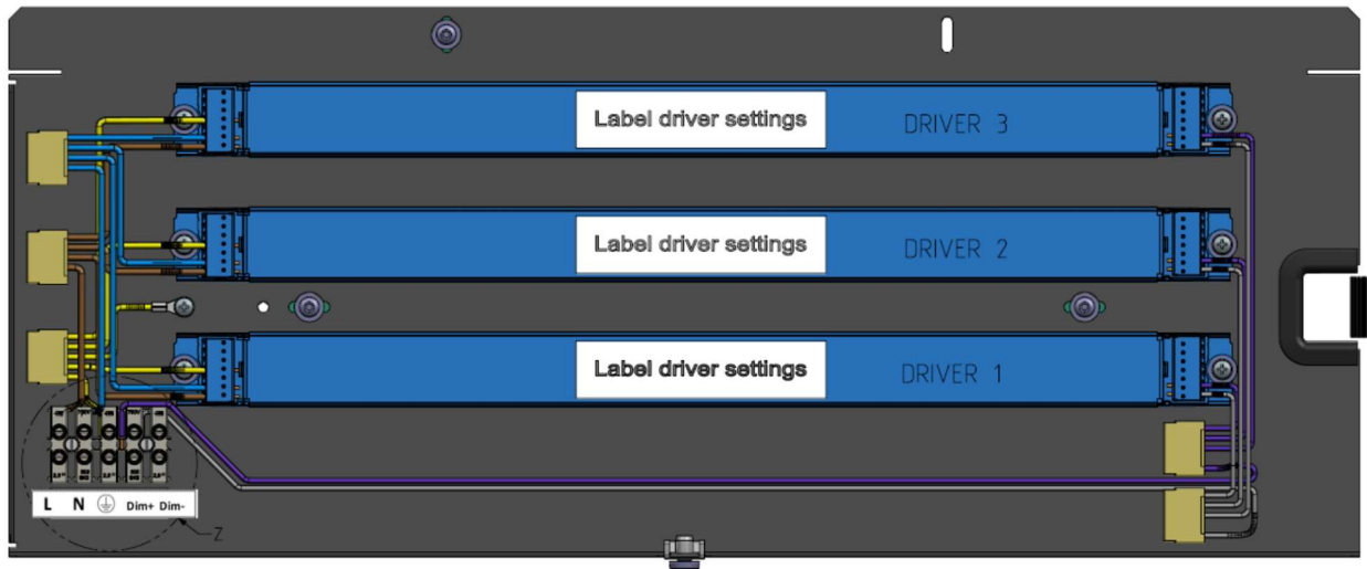
Figure 2: Inside look of an E-box with the maximum quantity of drivers
