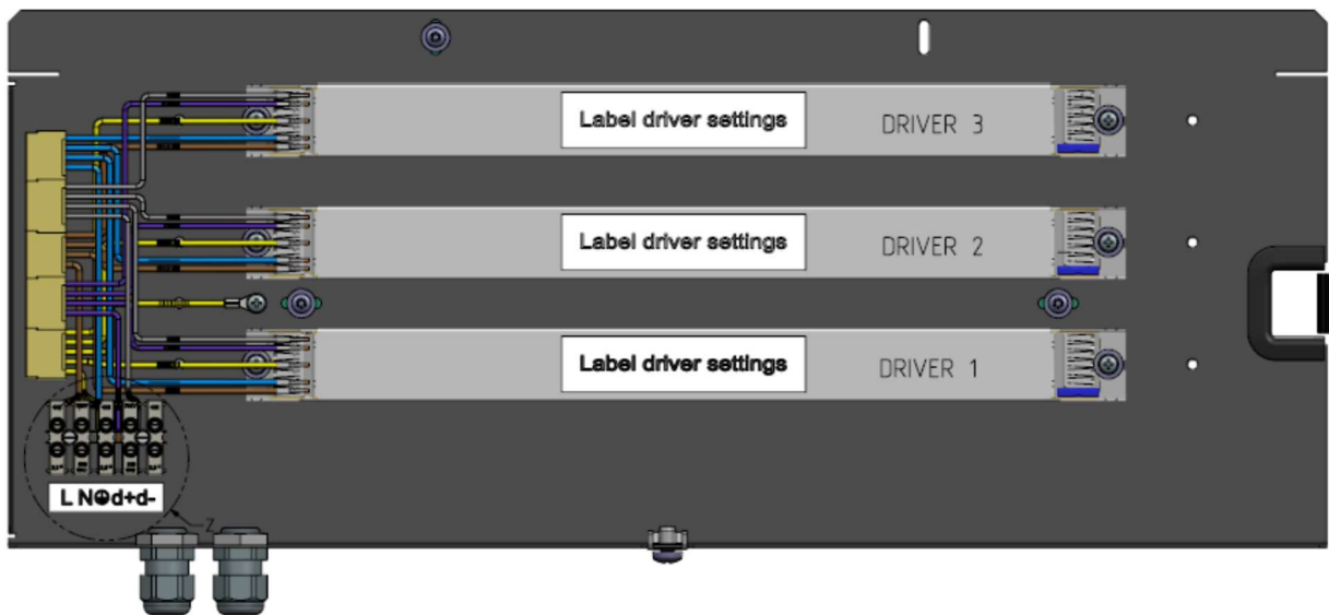
Figure 1: Inside look of an E-box with the maximum quantity of drivers
