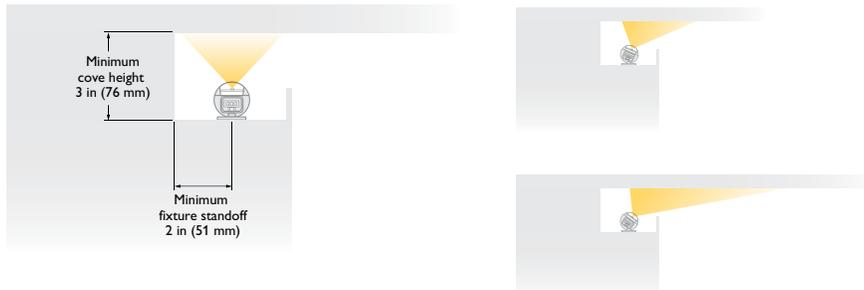
✳️ This diagram provides general guidelines for positioning iColor Cove EC Powercore fixtures in coves with matte white surfaces. Specific dimensions and positioning depend on the details of your installation.
