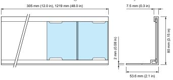
**Attaching Masking Plate**
