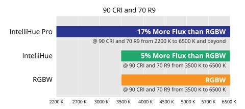
IntelliHue Pro and IntelliHue deliver more flux than RGBW. IntelliHue Pro excels across a wider range of color temperatures—particularly in critical color temperatures, including amber. And IntelliHue provides more flux in cooler color temps.
