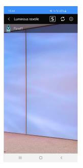
11 Tap "Panels in the network" to show all connected Luminous Textile panels. As a result, for each panel the IP address is displayed. The IP address can be used to connect to the panel via a web browser.
